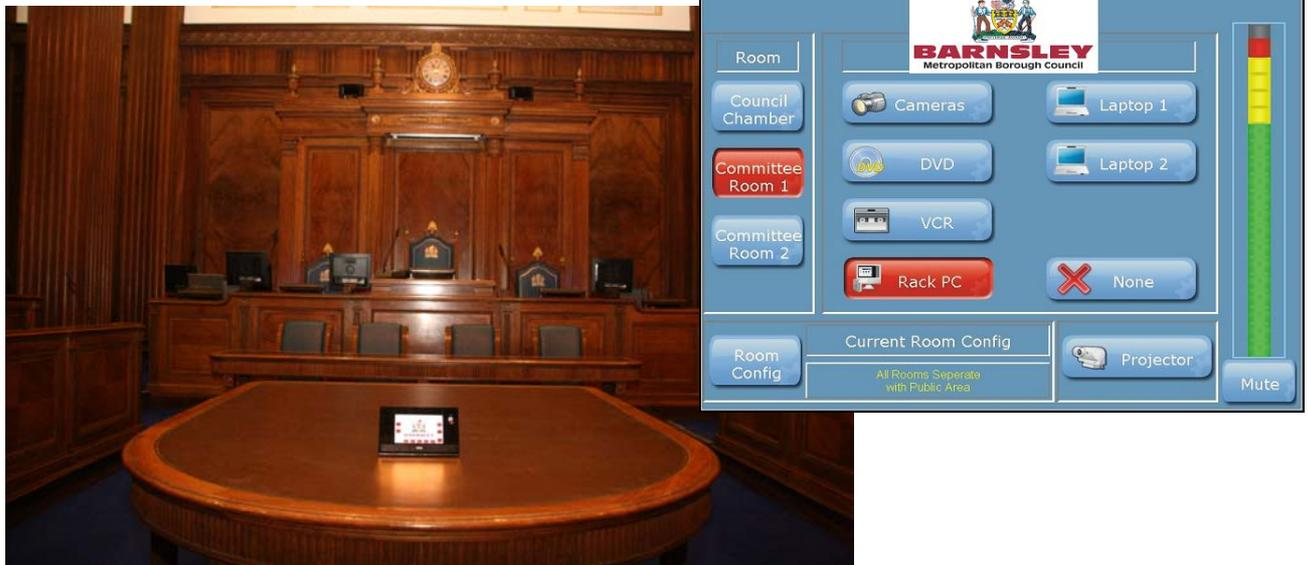
An AMX master touch screen unit has been programmed to operate all of the conference equipment. Projectors on/off, screen up / down, signal source select, volume control, webcast broadcast on / off and whole system on/off is all achieved by using the one touch screen
